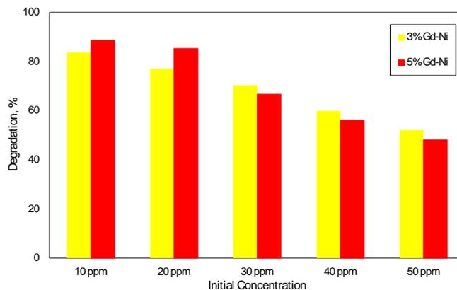
Figure III Effect of initial concentration on theophylline removal (pH: 7, catalyst dosage: 20g)
