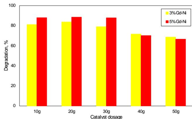
Figure II Effect of catalyst dosage on theophylline removal (pH: 7, initial concentration: 10 ppm)
