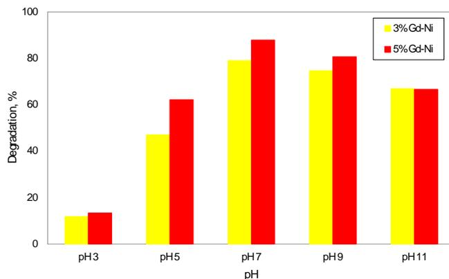
FIGURE I. Effect of pH on theophylline removal (catalyst dosage: 30g, initial concentration: 10 ppm)
