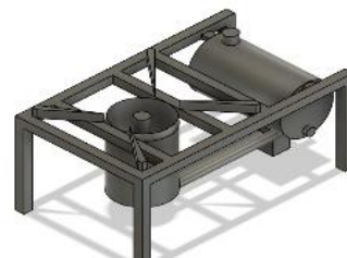
Figure 1. Design of used oil stove test equipment with additional heater
