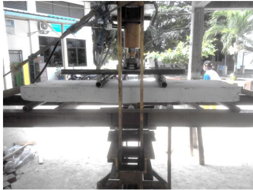
Figure 6. slab testing two point load
