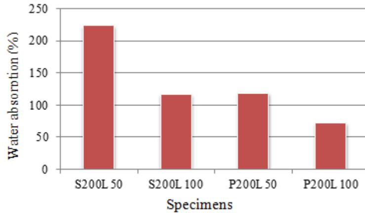
Figure 6. Test results for particle board water absorption
