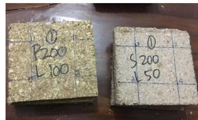
**Figure 3.** Particle board areca nut and Mahang wood powder
