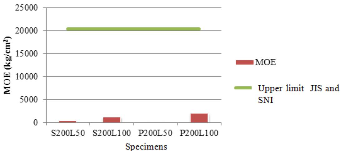
Figure 9. MOE test results for 4 specimens
