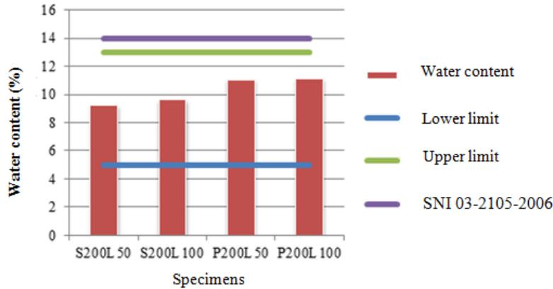
**Figure 4.** Test results for particle board water content
