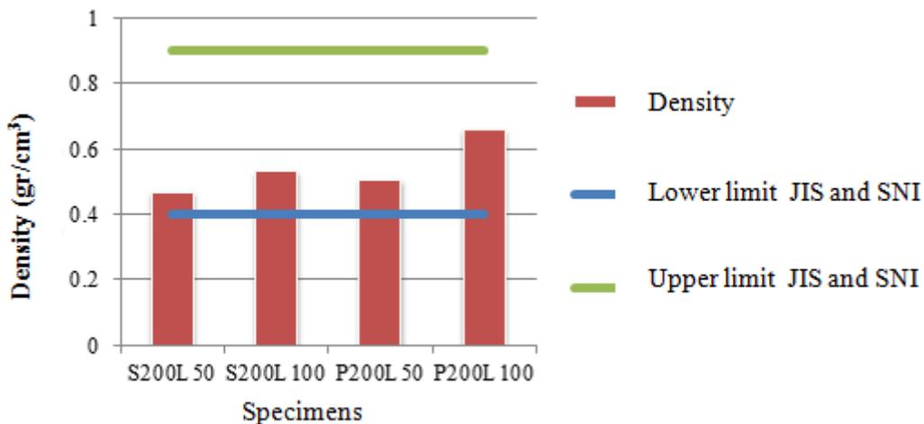
**Figure 5.** Test results for particle board density
