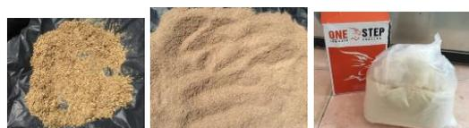
**Figure 1.** Particle board materials
