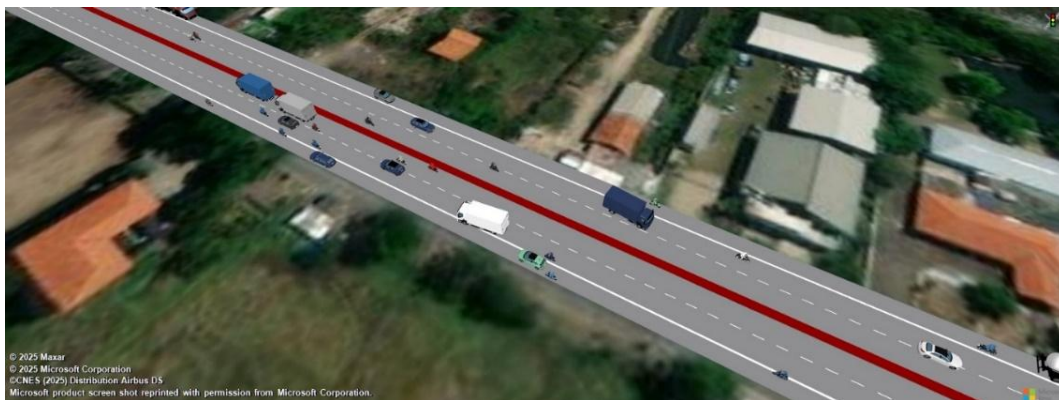
Figure 5. PTV VISSIM Microsimulation Model of the Study Section
