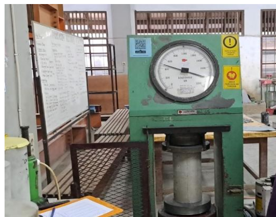
Figure 12. Testing Concrete Cylinder Compressive Strength
