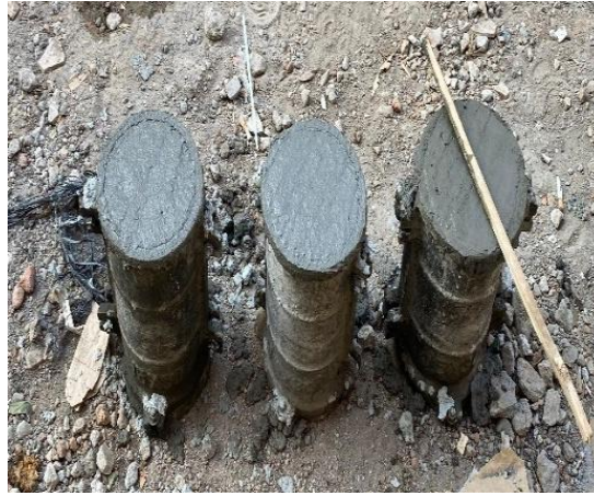
Figure 11. Levelling the surface of cylindrical test specimens
