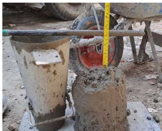
Figure 10. Measuring the Height of the Concrete Mix
